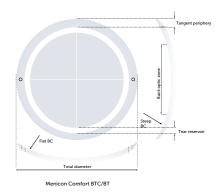
Note that the periphery is spherical (1 tangent).
